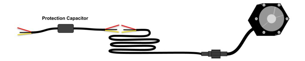
For dual color Pod Lights: Connect wires to a switch to toggle between the main (white) light and the accent (color) light. The main (white) light runs off the RED wire and the accent (color) lights run off the YELLOW wire. The BLACK wire is ground and can be wired to the ground pin of the switch or directly to the negative terminal of the battery.
